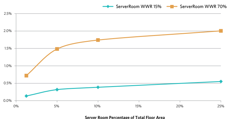
CHART 10.1 | ENERGY INCREASE PER FLOOR BY LOCATING 24-HOUR AIR-CONDITIONED ROOMS WITH THE EXTERNAL FAÇADE INSTEAD OF AT THE CENTER (CORE) OF THE BUILDING (WWR = WINDOW-TO-WALL RATIO)
