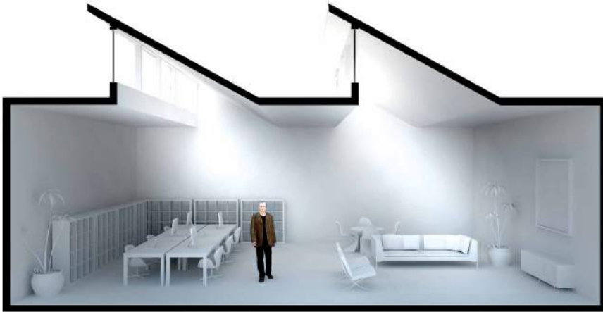
FIGURE 4.6.2 | TYPICAL SAW-TOOTH ROOF LIGHT DAYLIGHT HARVESTING
