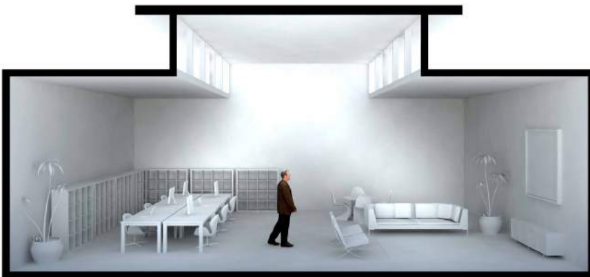
FIGURE 4.6.3 | TYPICAL ROOF MONITOR DAYLIGHT HARVESTING
