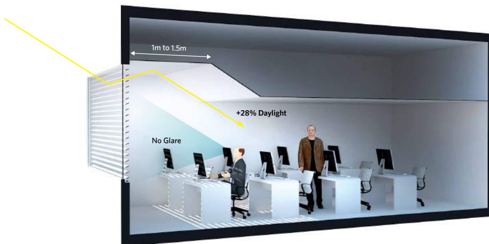
FIGURE 4.5.7 | DAYLIGHT ILLUMINATION LEVEL IS 28% HIGHER THAN FIGURE 4.5.6
