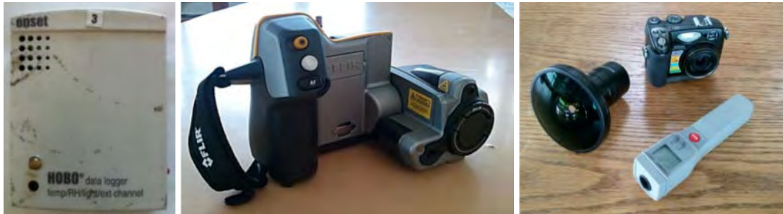
Figure 30 U12 HOBO Data Logger, FLIR Thermographic Camera, Fish Eye Camera (Patwardhan, 2012)
