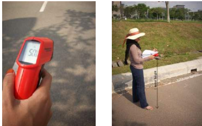
Figure 4.33 The reading taken from handheld Meterman IR608 Infrared Thermometer (left); and measurement procedure during measurement taken at 1m chest height
