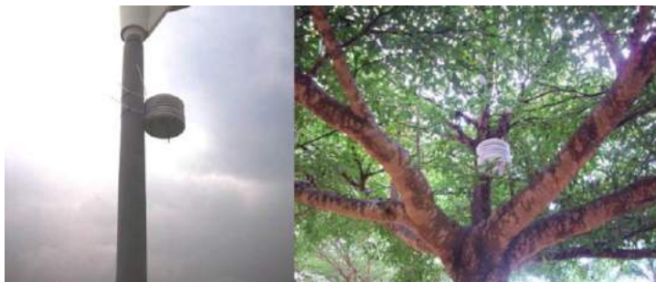
Figure 4.31 Tiny Tag installed in Stevenson screen attached to (left) lighting post, and (right) tree trunk
