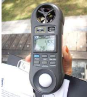
Figure 4.46 Lutron LM-8000 Portable 4 in 1 Anemometer, Hygrometer, Lux Meter and Thermometer
