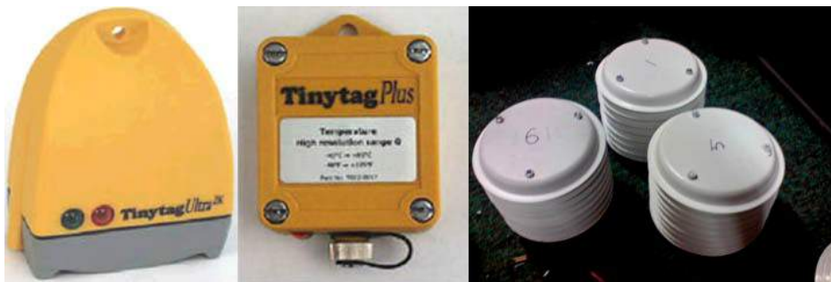
Figure 4.23 Tiny Tag TGP-4500 Ultra and TGU-4500 Plus portable data logger with Stevenson Screen
