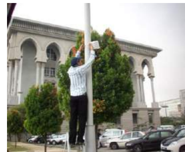
Figure 4.32 Installation of Tinytag instruments attached to lighting post at a height of 3m
