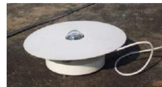
Figure 4.30 Pyranometer with base and screen model CM – CM 5
