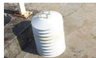
Figure 4.28 Vaisala temperature and humidity probe HMP35DGT with Stevenson screen
