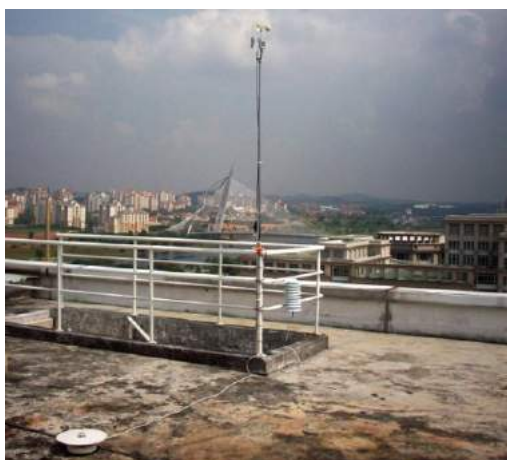
Figure 4.26 The weather station was set up at the edge of the 10m-high rooftop
